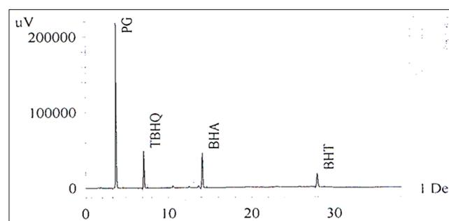
Fig. 1: Chromatogram of standard solution mix
