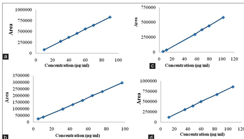
Fig. 2: Calibration curve of BHA,  $y=9385.2x-10263$  (a), BHT,  $y=5970.1x-31248$  (b), Propyl Gallate,  $y=29851x+50616$  (c), and TBHQ,  $y=7793.1x+27100$  (d)
