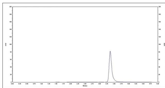
Fig. 4: Representative chromatogram of standard (10  $\mu$ g/ml)
