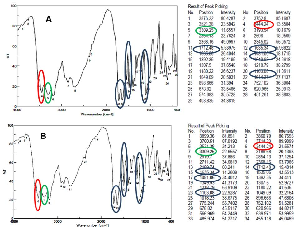
Fig. 3: Standard acyclovir (A) and sample infra-red spectra (B)
