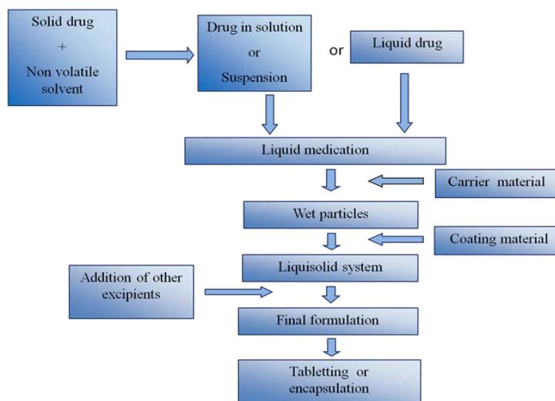
Fig. 7: General preparation procedure of liquisolid formulation [2]
