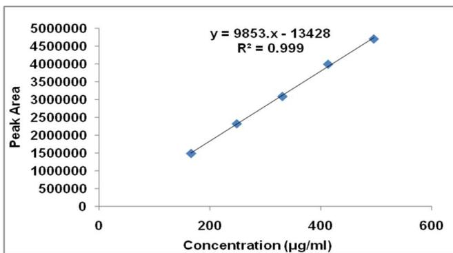
Fig. 5: Linearity chart for dosulepin hydrochloride
