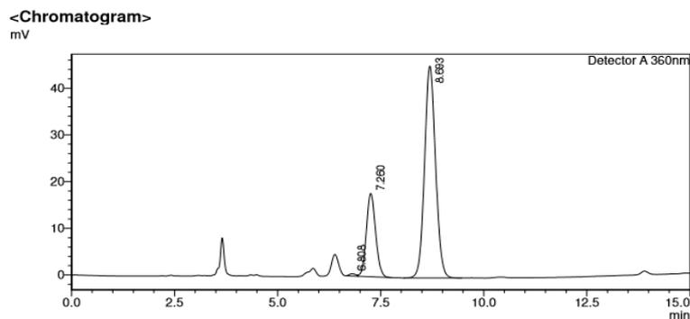
Fig. 2: Chromatogram of curcumin and piperine using optimum chromatographic conditions
