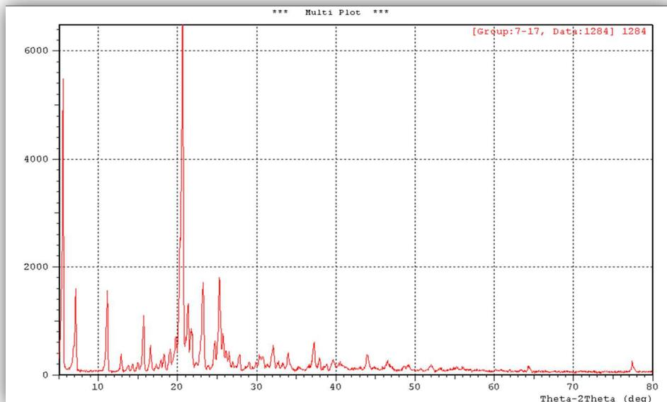
Fig. 18: Powder X-ray diffraction analysis of the selected formula F7
