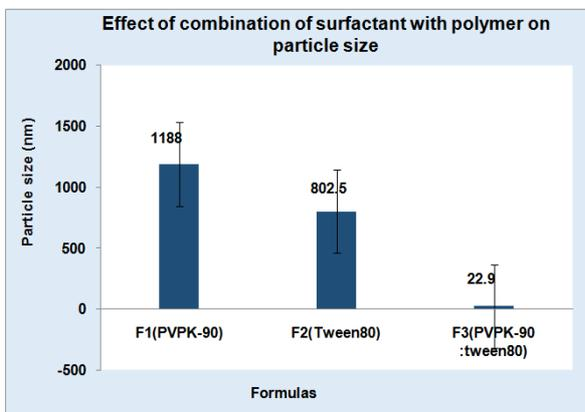
Fig. 3: Effect of a combination of the surfactant with polymer on the particle size of nanosuspension (n=3)
