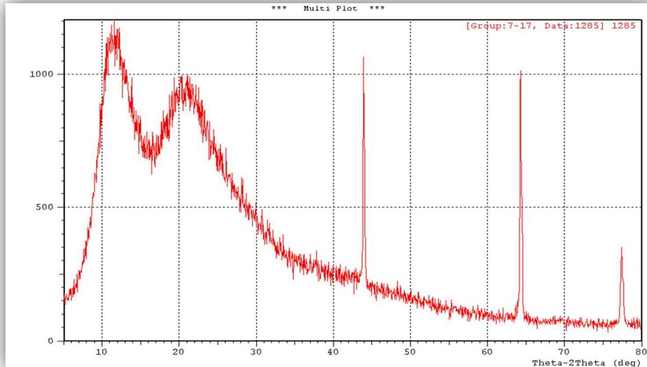
Fig. 17: Powder x-ray diffraction analysis of the PVP K-90
