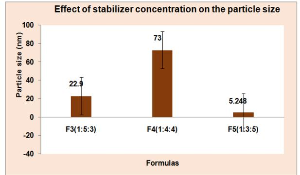
Fig. 4: Effect of stabilizer concentration on the particle size of nanosuspension (Results are expressed as mean, n=3)
