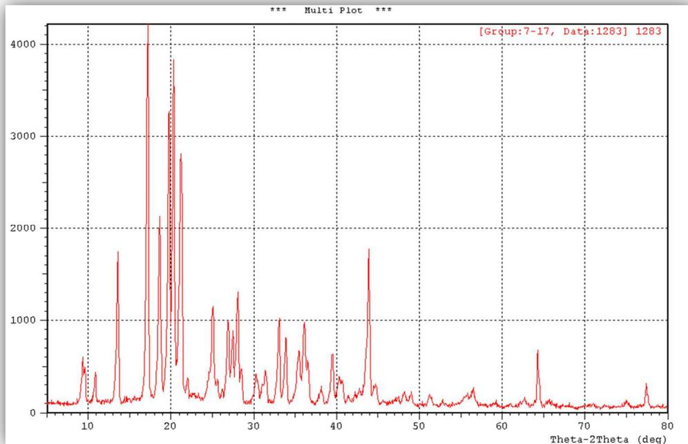
Fig. 16: Powder X-ray diffraction analysis of pure lafutidine
