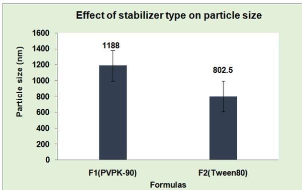
Fig. 2: Effect of stabilizer type on the particle size of nanosuspension (Results as an as mean, n=3)
