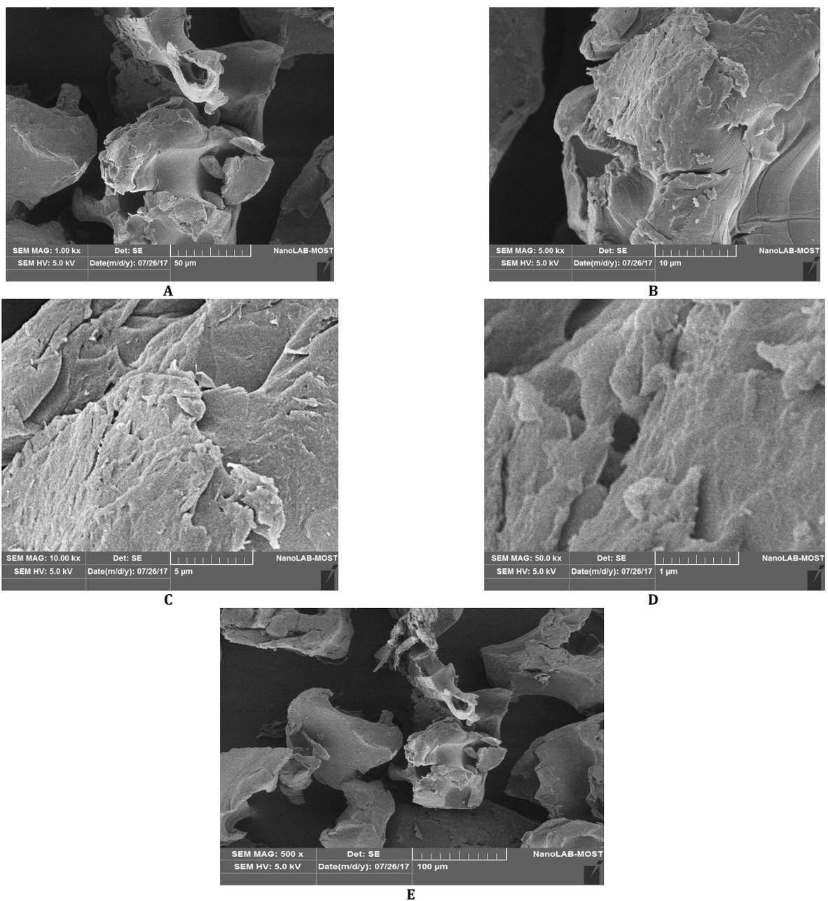
**Fig. 14: Scanning electron microscope of PVP K-90 (A, B, C, D, and E) at 1K, 5K, 10K, 50K and 500X magnification respectively**
