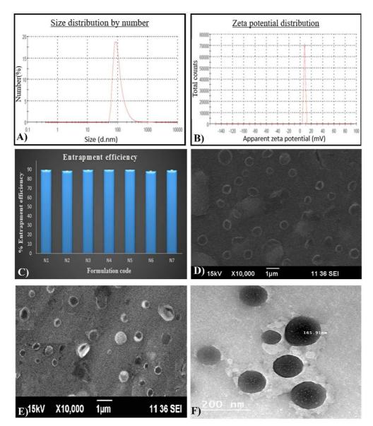
Fig. 2: (A)Vesicle size of niosomal midazolam(B) Zeta potential of niosomal midazolam(C) Entrapment efficiency of niosomal midazolam (D) SEM image of niosomal midazolam(E) SEM image of niosomal midazolam(F) TEM image of niosomal midazolam transdermal patch
