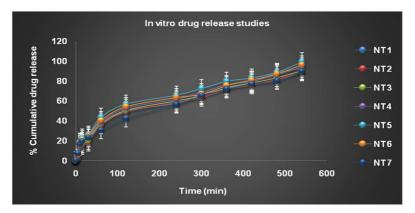
Fig. 5: In vitro release studies of different midazolamloaded niosomaltransdermal patch formulations, (values are expressed as mean±standard deviation, n=3)
