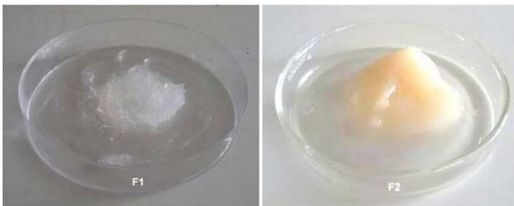
Fig. 7: The prepared gels F1 (carbopol 934) and F2 (xanthan gum) as gelling agents
