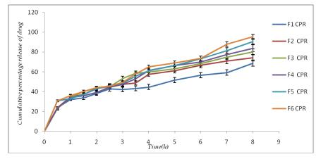
Fig. 3: Comparative C. P. R. of ibuprofen from solid dispersed matrix tablets (number of experiments, n = 3; data given in mean±SD)
