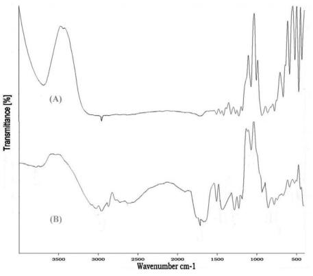
Fig. 1: FT-IR spectrum of-(A)-pure ibuprofen and (B)-formulation mixture
