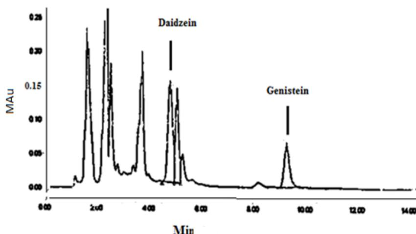
Fig. 1: Chromatogram of soybean samples obtained by HPLC using sun fire TMC-18 C18 column (150 mm x 4.6 mm, 5  $\mu\text{m}$ ). The mobile phase used was acetonitril: 0.1% acetic acid (35: 65), flow rate of 0.8 ml/min
