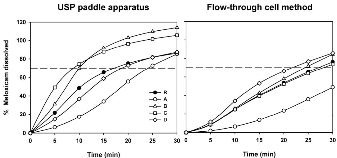
Fig. 2: Dissolution profiles of meloxicam reference (R) and generic formulations (A-D). The dashed line shows  $Q = 70\%$ . For clarity the error bars were omitted, mean,  $n = 12$
