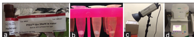
Fig. 3: (a and b) Addition of propidium monoazide and incubation in the dark. (c) Exposure with 600 W for 20 min. (d) Detection and quantification of DNA Enterococcus faecalis through real-time polymerase chain reaction
