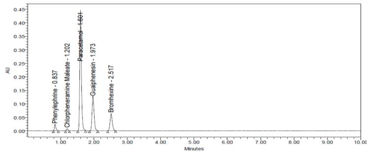
**Fig. 14: Chromatogram of peroxide degradation**
