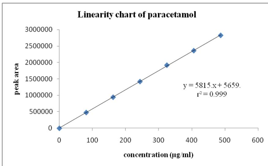
Fig. 9: Calibration plot of paracetamol
