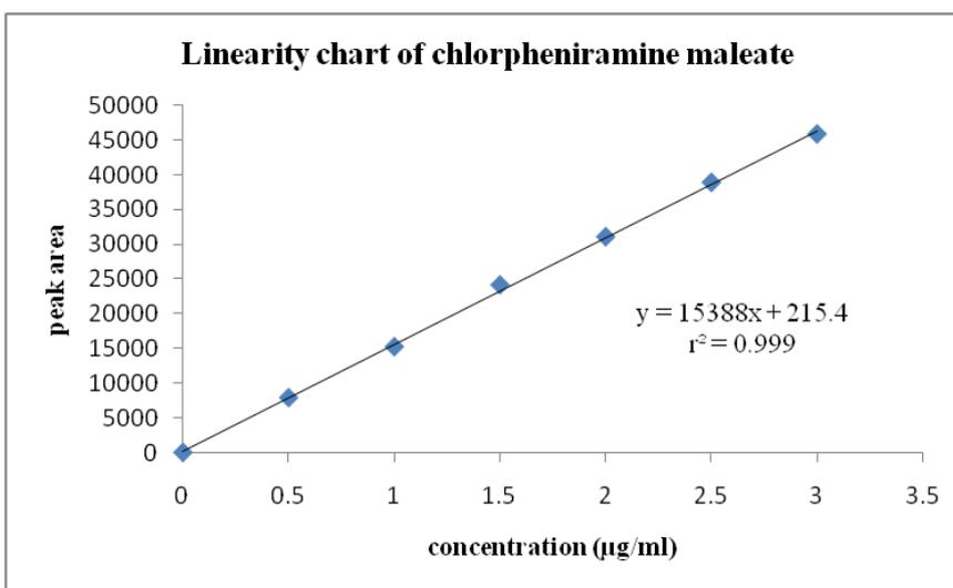
Fig. 8: Calibration plot of chlorpheniramine maleate
