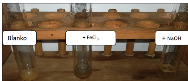
Fig. 2: The flavonoid and phenolic compound test of ethyl acetate extract of peanut shell
