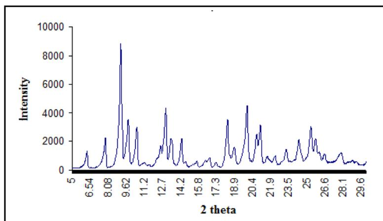
Fig. 3: X-ray diffractogram of gatifloxacin drug sample
