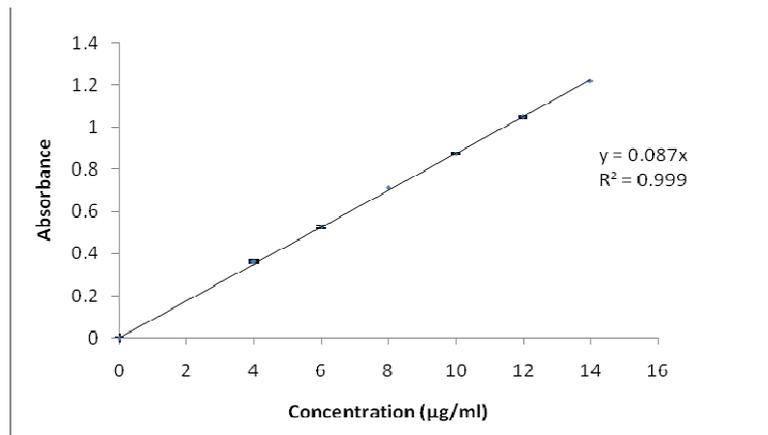
Fig. 4: Calibration curve of gatifloxacin in distilled water at 286 nm (mean±SD, n=3)
