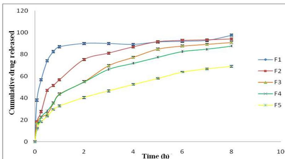
Fig. 9: *In vitro* drug release profile of gatifloxacin *in-situ* gel formulation in simulated lacrimal fluid (SLF) (mean±SD, n=6)
