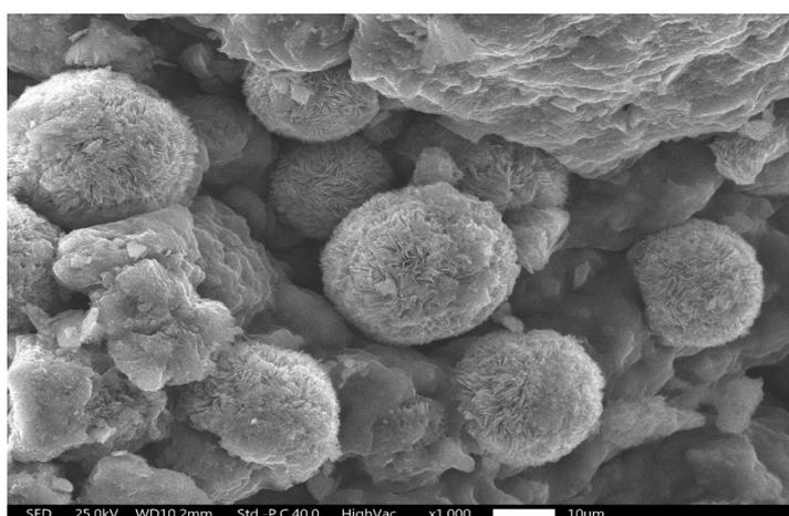
**Fig. 1: SEM observation of OX microspheres**
