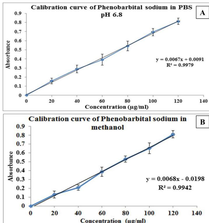
Fig. 2: (A) The standard calibration curve of the pure drug of Phenobarbital sodium in PBS pH 6.8 with slope, intercept and regression coefficient, (B) The standard calibration curve of the drug phenobarbital sodium in methanol with slope, intercept and regression coefficient, (Values are expressed as mean±standard deviation, n=3)
