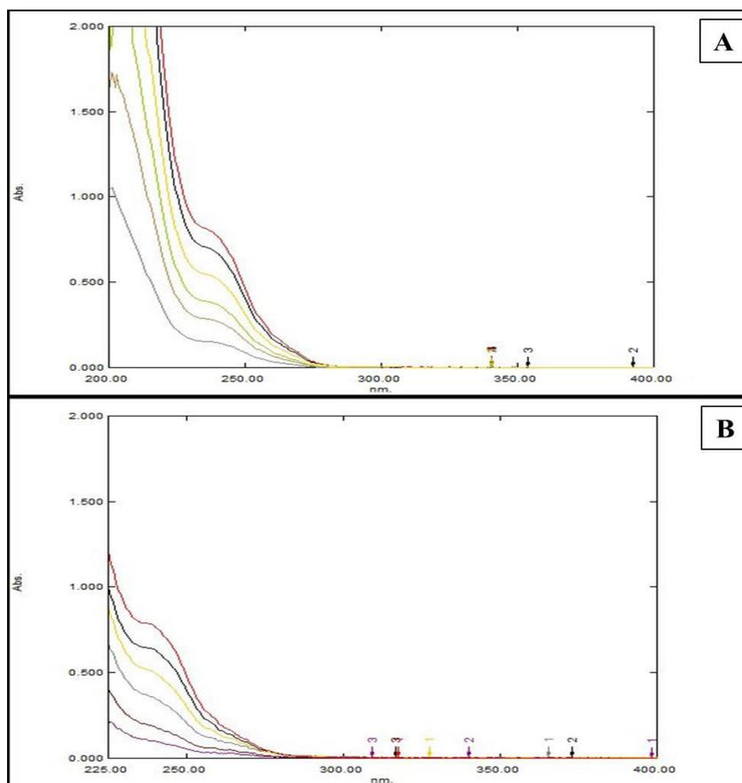
Fig. 1: (A) Absorption maxima of phenobarbital sodium in PBS pH 6.8, (B) Absorption maxima of Phenobarbital sodium in methanol
