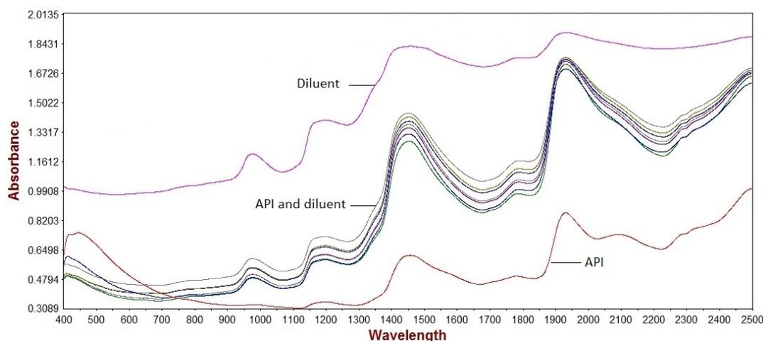
Fig. 2: NIR spectra of API, diluent and the powder blends of API and diluents
