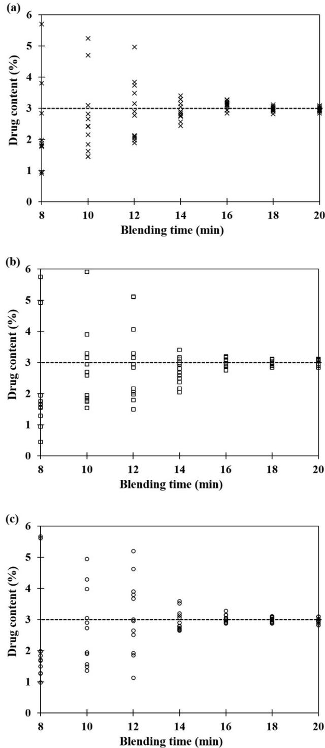
Fig. 4: The predicted API content between 8–20 min of blending process of (a) batch no. I, (b) batch no. II and (c) batch no. III (12 samples from each of the 12 locations), dot line represents the nominal API content (3%)
