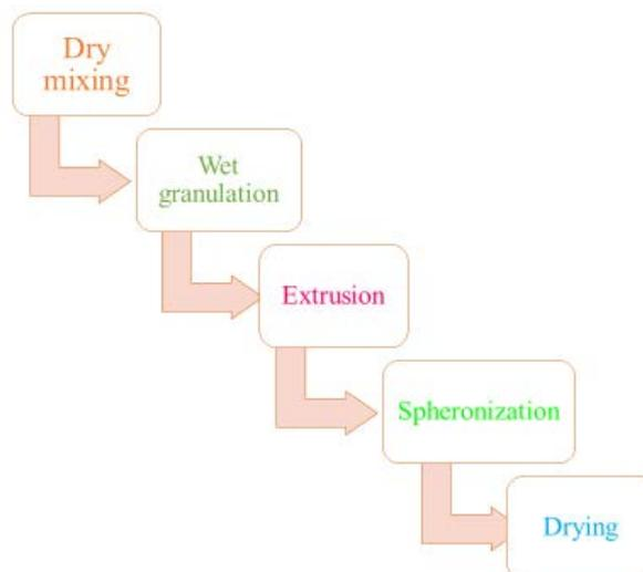
Fig. 4: Steps involved in manufacturing of pellets
