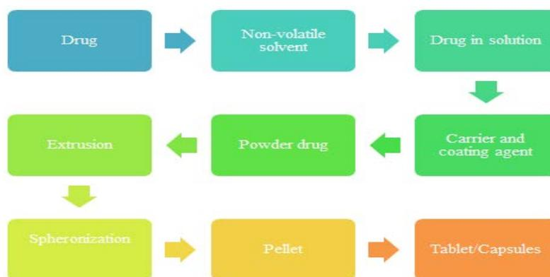
Fig. 3: Manufacturing steps involved in liquisolid-pellet technology
