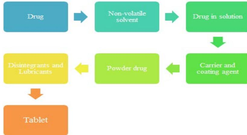
Fig. 1: Manufacturing steps involved in liquisolid technique
