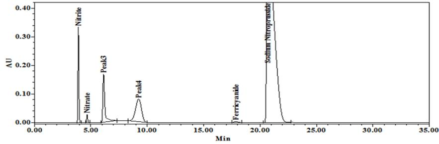
Fig. 8: Base degradation chromatogram of SNP injection formulation
