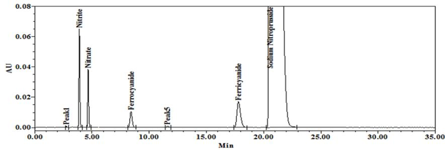
Fig. 10: Thermal degradation chromatogram of SNP injection formulation
