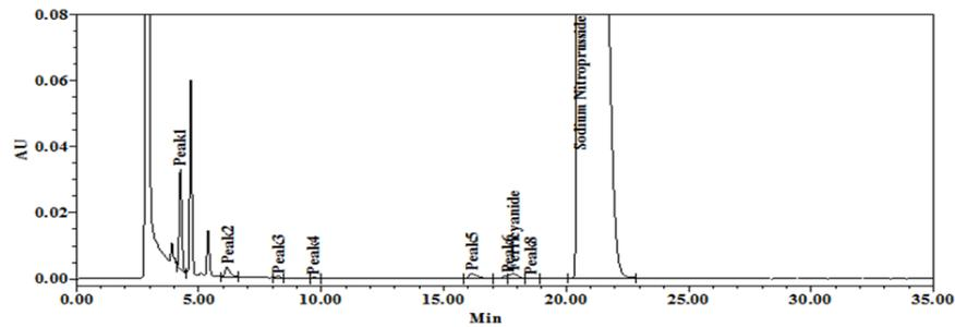
Fig. 9: Oxidative degradation chromatogram of SNP injection formulation
