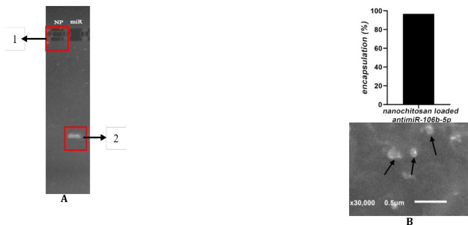
Fig. 1: (A) Agarose gel electrophoresis of chitosan/antimiRNA (1) Naked antimiR (2); (B) Efficiency of entrapment of the Ch-NP-antimiR-106b-5p as measured by NanoQuant and spherical morphology of nanochitosan was visualized by Scanning Electron Microscope, Abbreviation: Ch-NP-antimiR-106b-5p: Chitosan Nanoparticle antimiRNA-106b-5p
