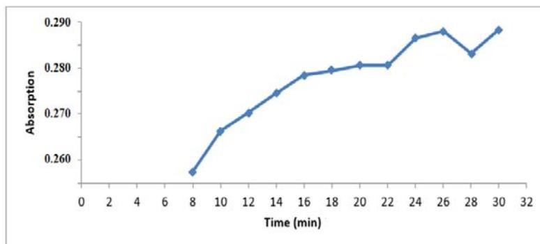
Fig. 2: The absorption profile of the standard cholesterol solution with Lieberman buchard reagent against time for 30 min
