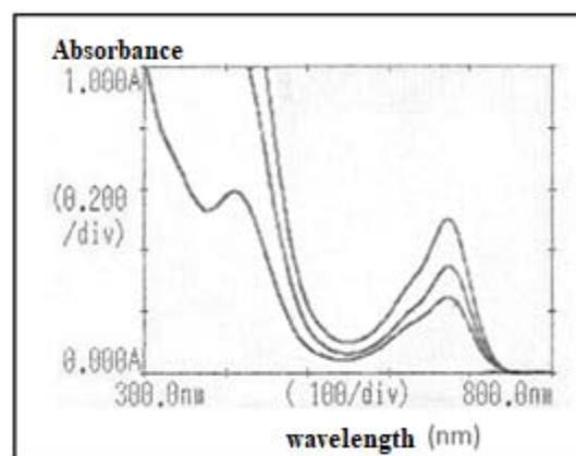
**Fig. 1: The maximum absorption wavelength of cholesterol standard solution**
