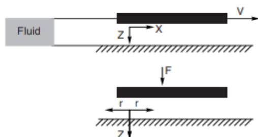
Fig. 1: Schematic representation of finger geometry as two parallel plates.  $V$ –finger velocity,  $Z$ –sample layer thickness,  $X$ –shear stress,  $F$ –shear force between fingers,  $R$ –finger radius [15]
