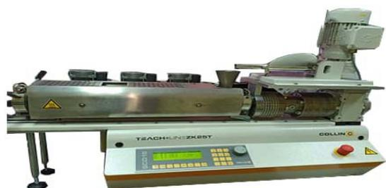
Fig. 4: Twin screw extruder
