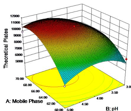
Fig. 4: Three-dimensional plot for theoretical plates as a function of pH of buffer and amount of methanol. Constant factor (flow rate-1 ml min<sup>-1</sup>)
