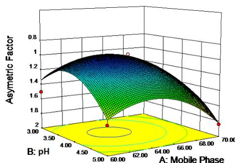
Fig. 3: Three-dimensional plot for asymmetric factor as a function of pH of buffer and amount of Methanol. Constant factor (flow rate-1 ml min<sup>-1</sup>)
