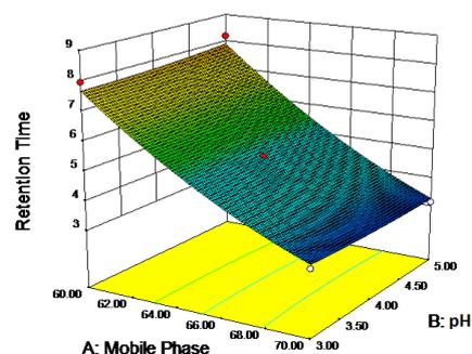
**Fig. 2: Three-dimensional plot for retention time as a function of pH of buffer and amount of methanol. Constant factor (flow rate-1 ml min<sup>-1</sup>)**
