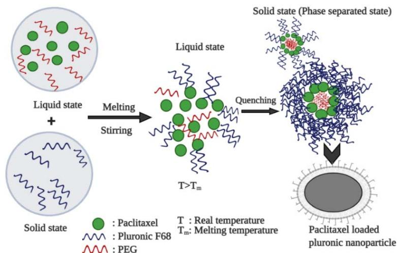
**Fig. 5: The formation of Pluronic-based NPs with a core/shell structure. The core is composed of a mixture of PEG (molecular weight: 400) and PTX (or DTX) and the shell is composed of Pluronic F-68 [151]**
