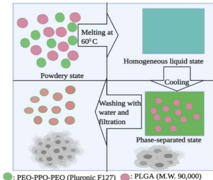
Fig. 6: Temperature-induced phase transition in the melt mixture of PLGA and Pluronic [153]
