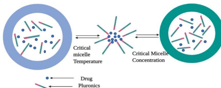
Fig. 3: The development of pluronic micelles in the watery medium according to Pluronics and temperature concentration [82]
