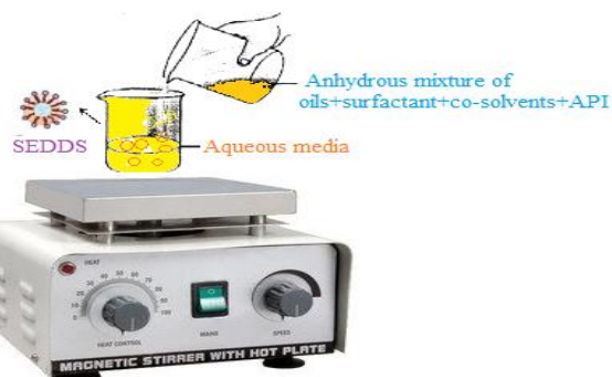
Fig. 4: SEDDS preparation using a magnetic stirrer
