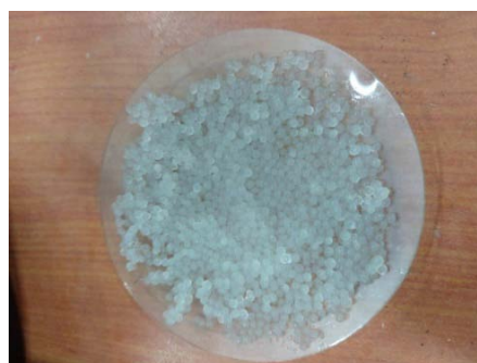
Fig. 2: Liposomes loaded eudragit coated alginate beads
