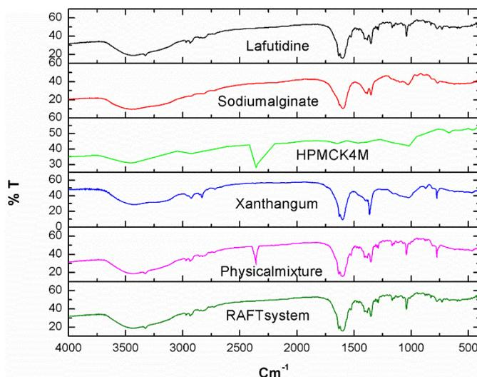
**Fig. 12: FTIR spectra of pure lafutidine, excipients, physical mixture, and lafutidine raft system**
