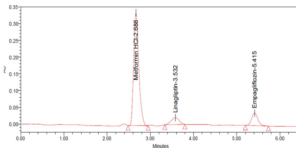
Fig. 11: Chromatogram of photodegradation study
