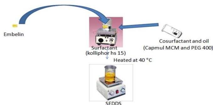
Fig. 1: Self-emulsifying drug delivery system preparation method
