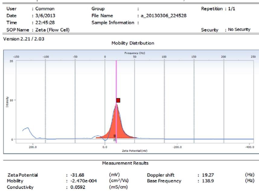
Fig. 5: Zeta potential of optimized embelin loaded SEDDS
