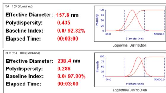
Fig. 2: Particle size of NLC and SLN dispersion
