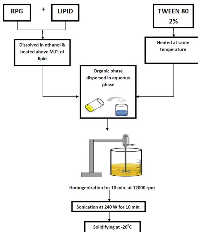
Fig. 1: Diagram of preparation of lipid-based dispersion (SLN and NLC)
