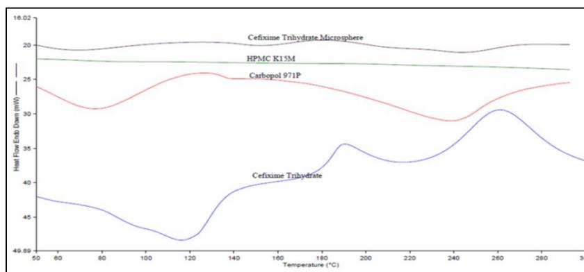
Fig. 10: Overlay graph of DSC analysis
