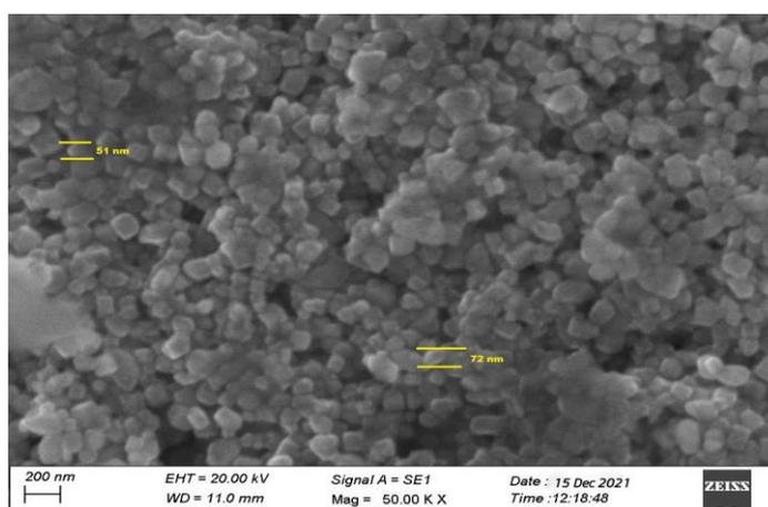
**Fig. 7: Analysis of nanoparticles by scanning electron microscopy (SEM), The dynamic light scattering measurement was done to find out how big the nanoparticles were. Laser diffraction showed that the size of the particles was between 40 and 120 nm**
