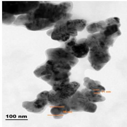
Fig. 9: Transmission electron microscopic (TEM) image of silver nanoparticles with Cluster in the range between 11 to 38 nm
