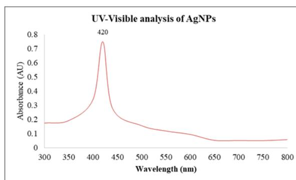
**Fig. 5: Analysis of the UV-Vis spectrum of AgNPs**
