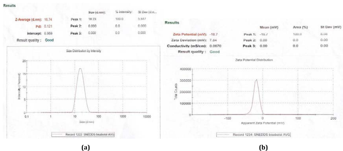
Fig. 1: Result of (a) Particle size analysis and (b) Zeta potential analysis
