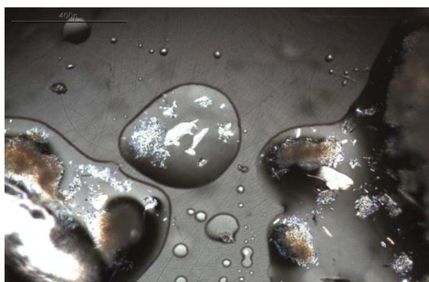
(B) Melting at 136 °C (Magnification: 10X)
