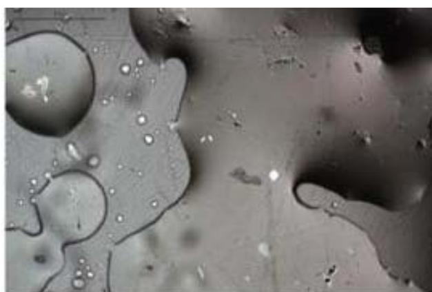
B) Melting at 174 °C (Magnification: 10X)
