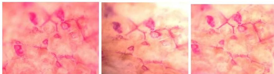
Fig. 10: Microscopic Image of pierced porcine skin using fabricated microneedles observed at 40X
