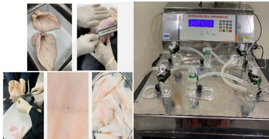
Fig. 2: Preparation of porcine skin samples and mounting on modified franz diffusion assembly
