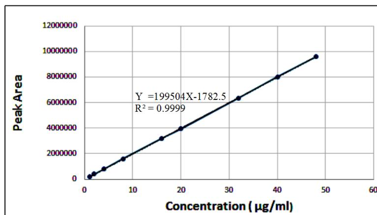
Fig. 3: Standard calibration curve of Famotidine at  $\lambda_{\max}$  254 nm
