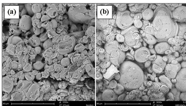
Fig. 4: SEM photographs of 40 mg loading famotidine floatable microspheres; Drug: alginate microspheres, and (b) Drug: alginate: GMO microspheres
