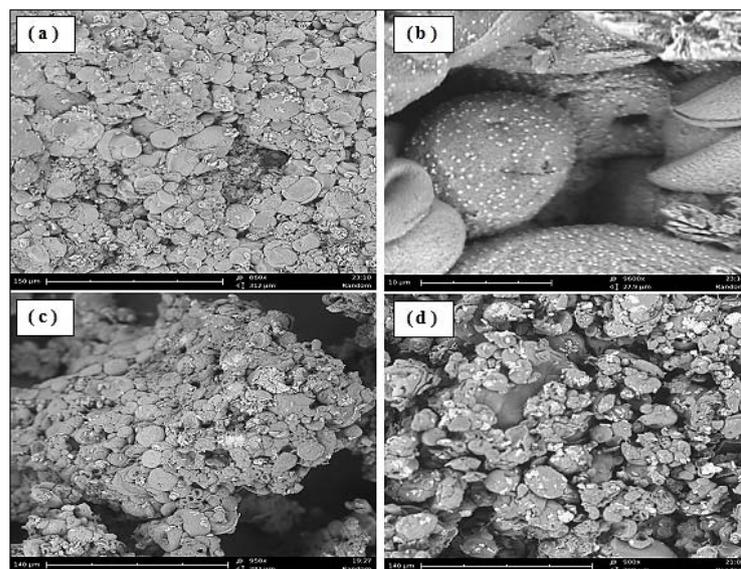
Fig. 2: SEM photographs of; (a and b) 1:0.25 w/w Alginate: GMO microspheres, (c) 1:0.5 w/w Alginate: GM O microspheres, (d) 1:1 w/w Alginate: GMO microspheres
