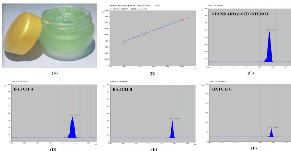
Fig. 1: (a)  $\beta$ -sitosterol hair gel formulation; (b) Calibration curve of  $\beta$ -sitosterol in HPTLC; (c) HPTLC chromatogram of standard  $\beta$ -sitosterol; (d) HPTLC Chromatogram of Batch A; (e) HPTLC chromatogram of Batch B; (f) HPTLC chromatogram of Batch C
