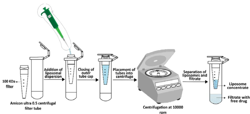
Fig. 2: Schematics of centrifugal ultrafiltration method
