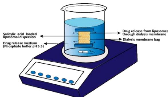
Fig. 3: Schematic diagram of *in vitro* drug release study
