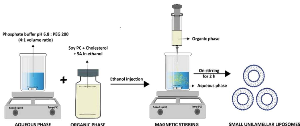
Fig. 1: Schematic diagram of the ethanol injection method
