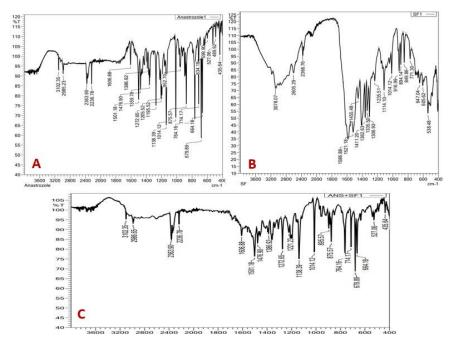
Fig. 1: FT-IR spectrums of (A) pure ANS, (B) silk fibroin, (C) SF-ANS-NPs-1
