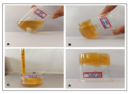
Fig. 8: SF-ANS-NPs-1 loaded *in situ* gel formulation A. at room temperature and B. after temperature increases (≥37 °C). C. Noted temperature at gelling point and D. inverted beaker after gelation
