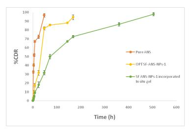
Fig. 2: Release profile of pure ANS, optimized SF-ANS-NPs-1 and SF-ANS-NP loaded in situ gel, (mean±SD, n = 3)
