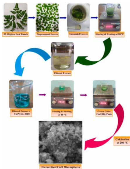
Fig. 5: Process of hierarchical CuO microspheres synthesis by M. oleifera leaves extract [44]
