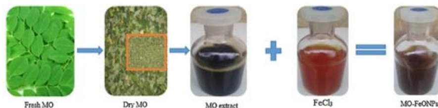
Fig. 6: Schematic representation the synthesis of MO-FeO [56]
