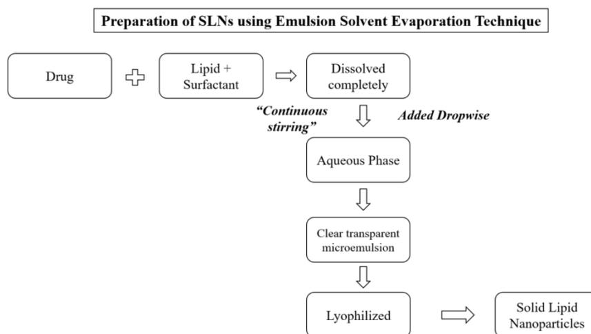
Fig. 3: Schematic representation of emulsion solvent evaporation technique [31]
