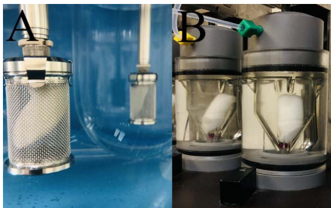
Fig. 2: Image of the dissolution of the reference formulation after 60 min using the USP Apparatus 1 (A) and 4 (B). The ovules only slightly modified their original shape
