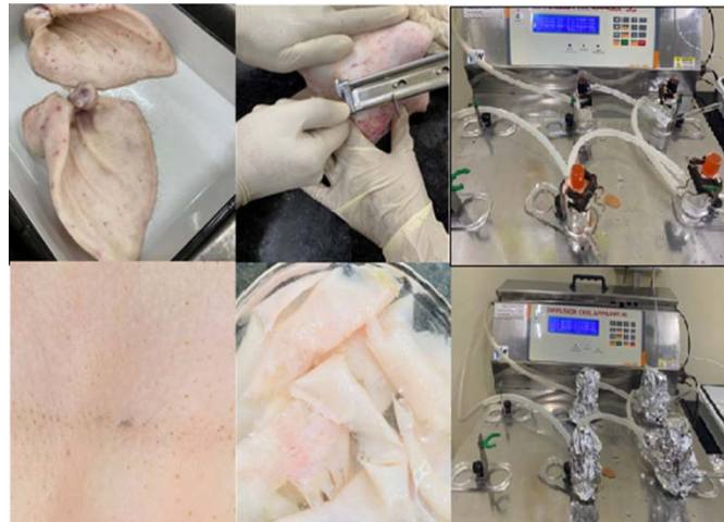
Fig. 3: Mounted porcine skin samples for permeation studies using a franz diffusion cell
