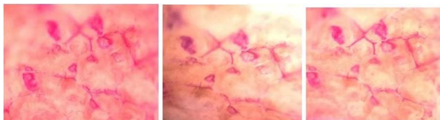
Fig. 10: Using fabricated MN, a Microscopic Image of poked pig ear skin
