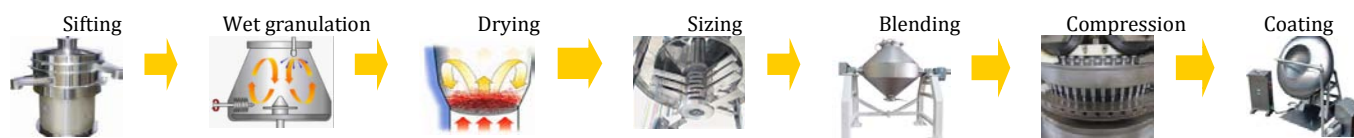
Fig. 2: Process flow for preparation of conventional film-coated ticagrelor tablets
