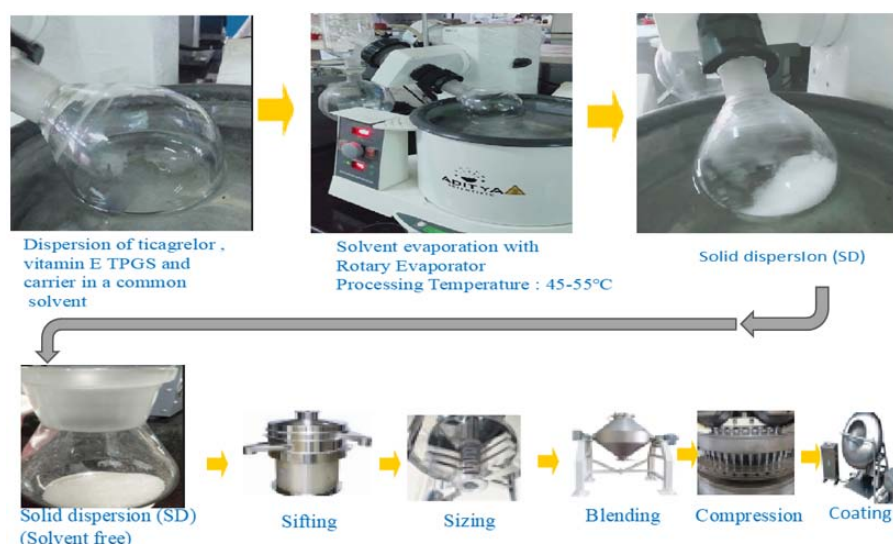
Fig. 3: Process flow for preparation of film-coated ticagrelor tablets with solid dispersion technology
