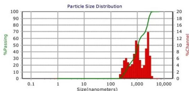
Fig. 2: Particle size analysis by dynamic light scattering technique
