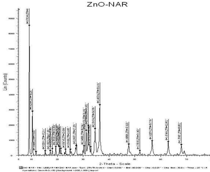
Fig. 3: XRD pattern depicting d values varying with 2θ range from 0° to 80°
