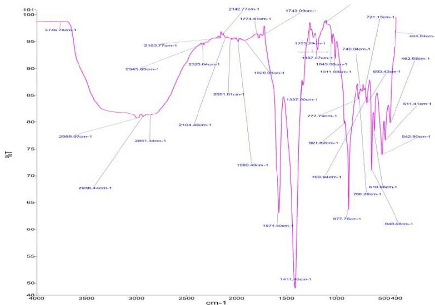
Fig. 4: FT-IR spectrum of naringin-loaded ZnO NPs
