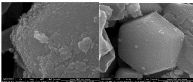
Fig. 5: HR-SEM images of naringin-loaded ZnO NPs at 60,000 X magnification
