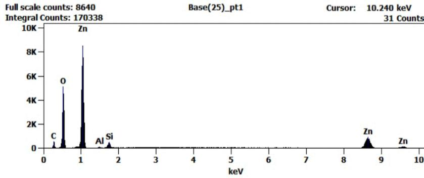
Fig. 7B: EDX elemental analysis of the naringin-loaded ZnO NPs
