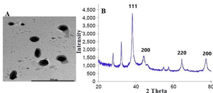
Fig. 3: (A) TEM analysis of AgNPs (B) XRD pattern of synthesized AgNPs
