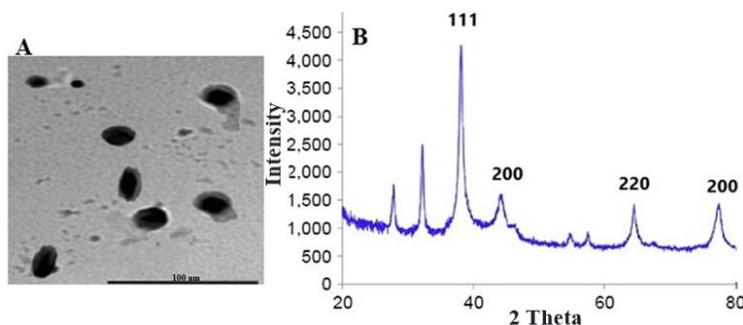
Fig. 3: (A) TEM analysis of AgNPs (B) XRD pattern of synthesized AgNPs
